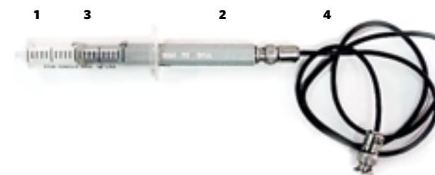
Fig. 2. Structure of ultrasound syringe using standard medical devices: 1 — syringe body; 2 — ultrasonic source IUT 0.88-1.03 F; 3 — sealing ring-cuff; 4 — cable for connecting the emitter with a medical ultrasound generator UZT-1.01 F
